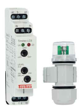
The Timetec-LCS controls lighting on the basis of ambient light intensity. It is used for switching street and garden lighting, illumination of advertisements and shop windows, etc. at night. The level of ambient light intensity is monitored by an external sensor and output is switched according to the level set on the relay.
